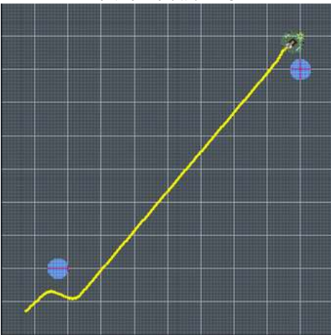
Fig. 8. Scenario 1: path planning with 2 obstacles in the unknown environment with self tuning FLC by SOM
