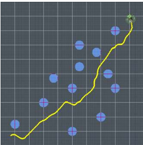
Fig. 7. Scenario 3: path planning with 12 obstacles in the unknown environment with FLC
