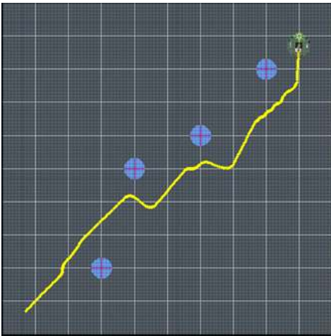
Fig. 6. Scenario 2: path planning with 4 obstacles in the unknown environment with FLC
